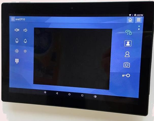
**The CP-11** 10" Android Intercom Monitor Control Panel is a multi-touch panel to control your video intercom. It is for use within a building. The use of IP technology and SIP protocol gives the intercom various options for connection to telephone systems. You can truly experience the perfect life of "intelligent community" and "smart home".
